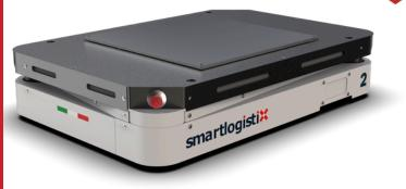
The AMR-X is a platform-type mobile robot available with several mounting options. Each attachment allows for a customized application. From bins to pallet holdings, to roller conveyors or transport chains, this robot is ideal for moving parts between different zones of a facility. The robot comes with a standard lifting system to drive underneath a loading unit, lift it up and transport it.
