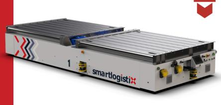
The OMNI Flex is an advanced mobile platform designed with scalable design to allow loads of up to 25 tons. Its omnidirectional navigation ensures exceptional maneuverability. OMNI Flex is offered with various options to carry different products, batches or frames. It can optionally offer lifting, tilting or customized actuator controls.
